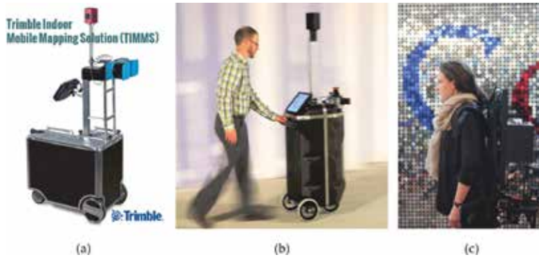
Figure 11. Indoor mapping systems: TIMMS (a), iMMS (b) and CARTOGRAPHER (c). Images courtesy of Trimble, SmartGeometrics and Google, respectively.
