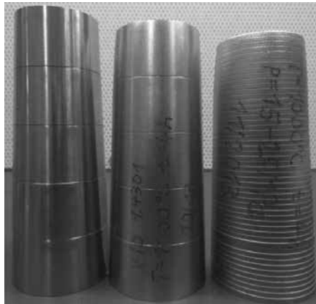
Figure 21. Conical samples made of 1.4301, T = 1000^{\circ}\text{C} , t = 4\text{ h} , F = 17.55\text{ kN} , corresponding to 15–25 MPa. Left: Before diffusion welding. Middle: Five segments, deformation: 5.41 and 5.11%, respectively. Right: Sample made of 51 layers; deformation: 8.34% [6].
