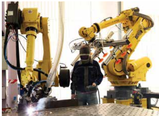
Figure 19. Robot-based HLAW machine on the base of 25 kW fiber laser.
