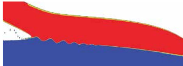
Figure 10. Eulerian simulation showing the development of wavy pattern at the welded interface.
