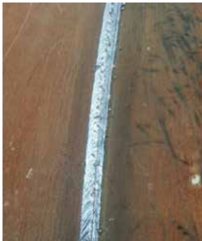
Figure 21. Root pass side. Orbital pipeline hybrid welding with 2 mm gap and 3 mm vertical displacement.
