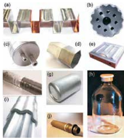
Figure 1. EMPT for industrial applications implemented by “PSTproducts” (a) Al/Cu electric bus bar [www.pstproducts.com], (b) EMPT crimped gear box part [www.pstproducts.com] (c) EMPT welded Al pressure vessel for air conditioning system [28], (d) EMPT welded Al/steel crash box [www.pstproducts.com], (e) EMPT welded Al/Cu cooling plate [www.pstproducts.com] (f) EMPT crimped Al/steel tube instrumental panel beam [28], (g) EMPT for hemming of a Al pressure vessel [28], (h) EMPT crimped Al lid on a pharmaceutical glass bottle [29], (i) EMPT crimped drive shaft [28] and (j) EMPT crimped air suspension [28].
