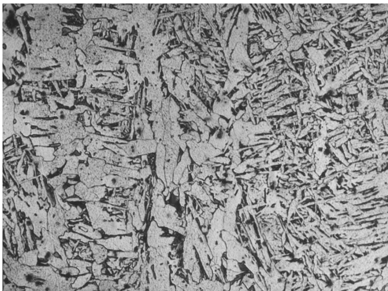
Figure 25. Weld, Nital Etch, magnification 250×, ferritic-pearlitic dendritic structure.
