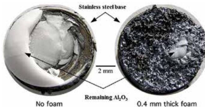
Figure 14. Fracture surfaces of joints without and with metallic foam following thermal cycling between 200 and 800 °C in air. Number of cycles to failure were <1 and 60 \pm 4 for samples without and with a foam interlayer, respectively [51].
