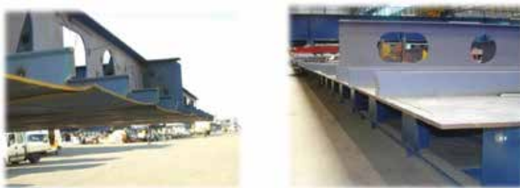
Figure 23. Comparison of MAG welded ship body section (left) with HLAW case (right).
