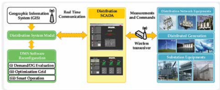
Figure 5. Architecture of the developed system.
