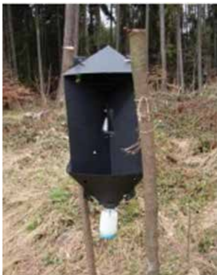
Figure 20. Pityogenes chalcographus wing trap installed in forest (own photo on experimental plots).
