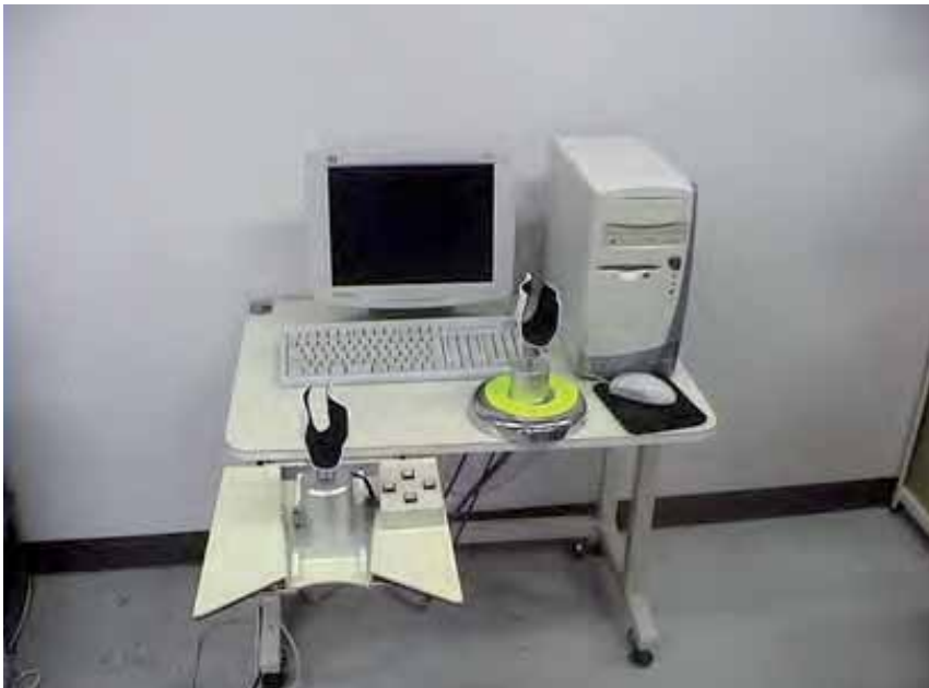
Fig. 1. The first and second prototype of upper limb rehabilitation system for spinal cord and peripheral nerve injury. The first prototype in the front left is mounted on a stage to place on the laptop. The second prototype is for desktop use.
