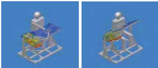
Fig. 23. Quasi-3-DOF rehabilitation system “PLEMO”: Horizontal state (left) and slanted state (right).
