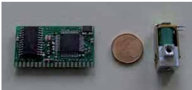
Fig. 4. Electric valve and control unit.
