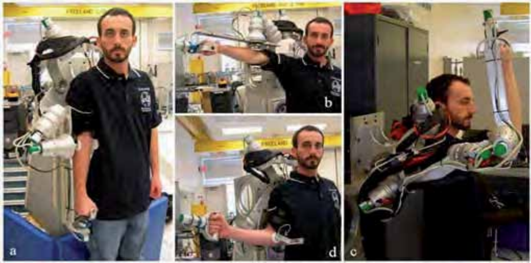
Fig. 4. Exoskeleton shown at (a) full shoulder adduction (b) 90 degree shoulder abduction, (c) mid-elbow flexion, and (d) near full lateral rotation.
