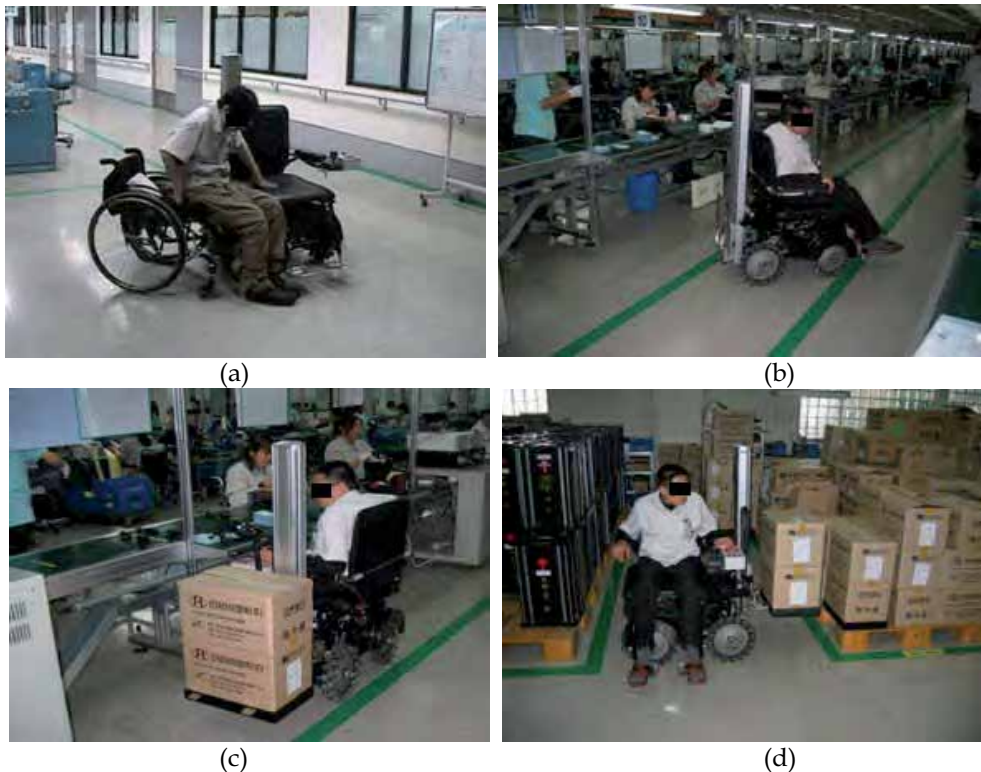
Fig. 20. User trials for Work Assistive Mobile Robot System Type II; (a) Transferring boxes, (b) Moving around, (c) Working at a desk, (d) Moving boxes.
