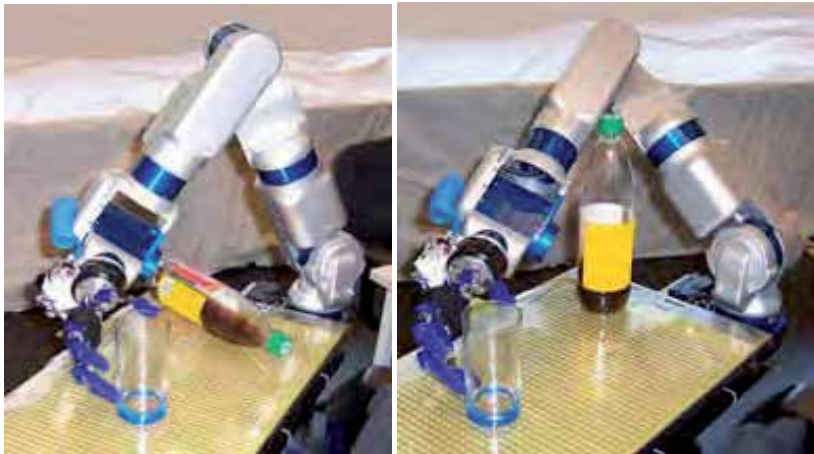
Fig. 17. Example of dexterous manipulation: a 6-joint arm can’t grasp a glass without collision with a bottle (left); by controllable movement of elbow it will be possible (right).
