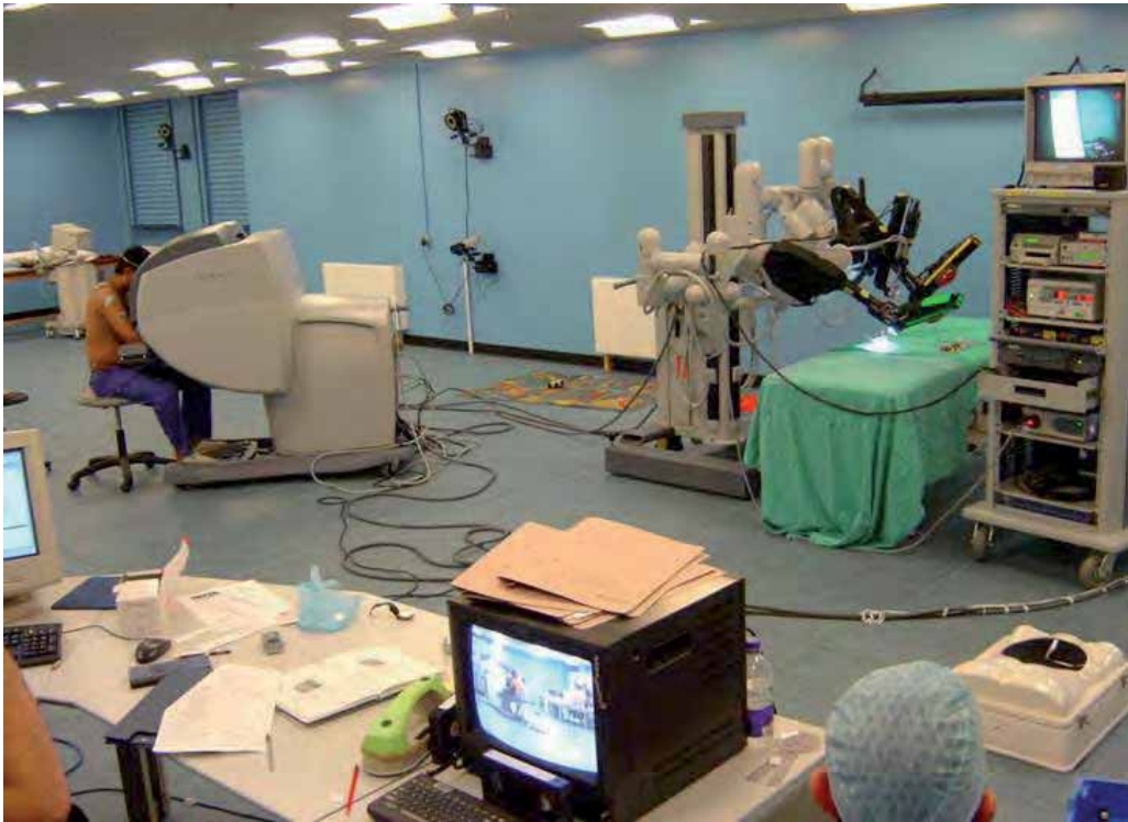
Fig. 1. Ergonomic assessment of da Vinci system in Gait Lab.
