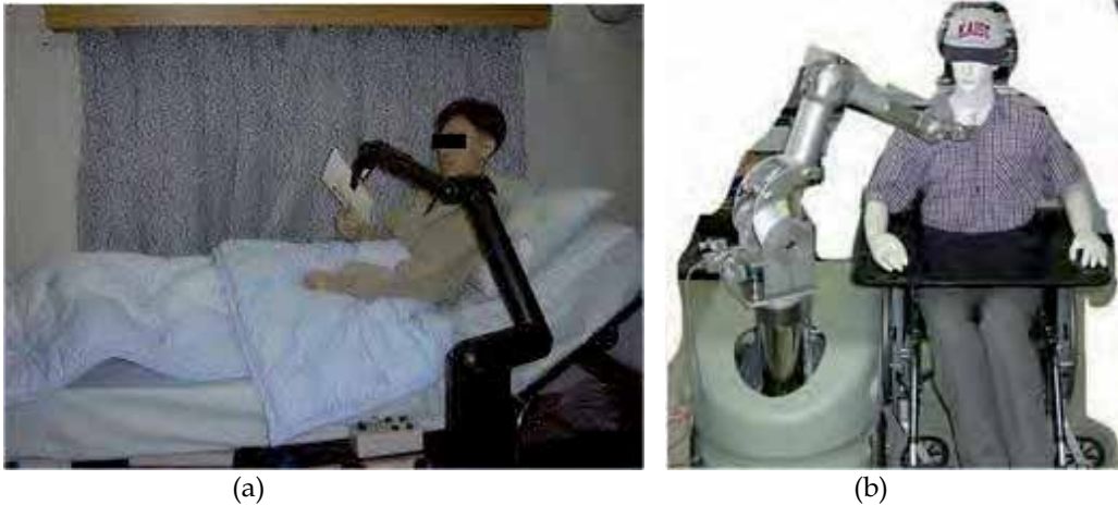
Fig. 1. Examples of robots for daily activities of the disabled; (a) Intelligent bed-robot system, (b) KARES II.
