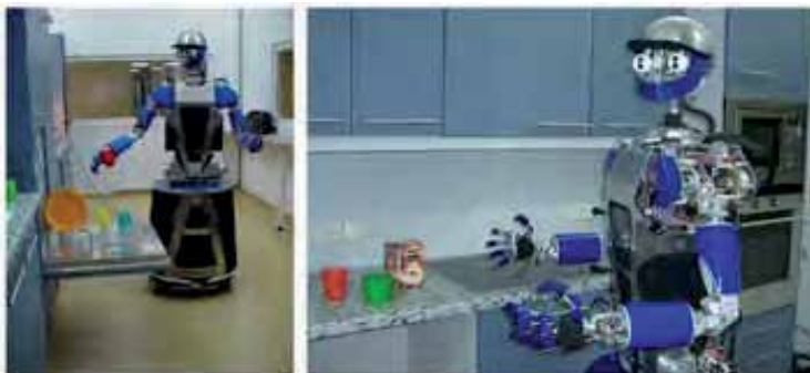
Fig. 6. The humanoid robot ARMAR-III in the demonstration environment (kitchen). The robot consists of seven sub-systems: head, left arm, right arm, left hand, right hand, torso, and a mobile platform.
