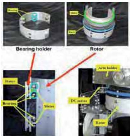
Fig. 2 Mechanism for shoulder inner/outer rotation motion assist.
