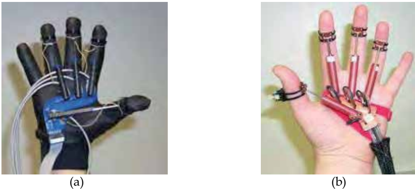
Fig. 3.2. (a) The Rutgers Master II force feedback glove, (b) The Rutgers Master II-New Design glove. Copyright Rutgers University.
