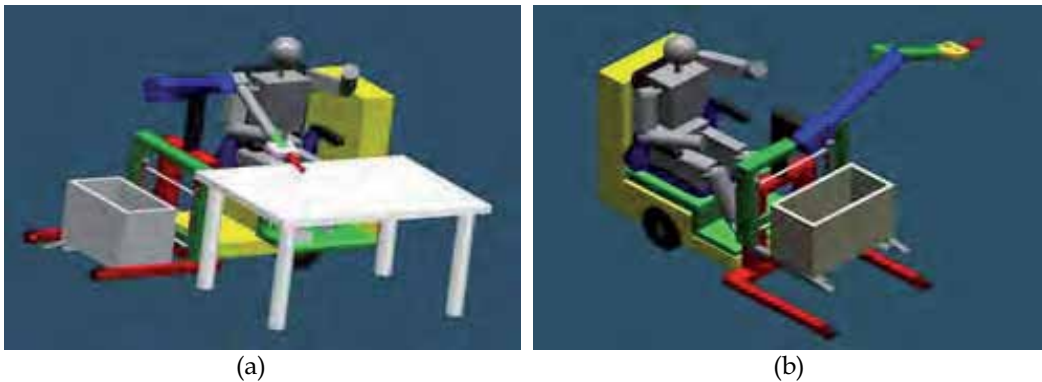
Fig. 11. Basic concept of work assistive mobile robot system type I; (a) assisting table tasks, (b) moving objects.
