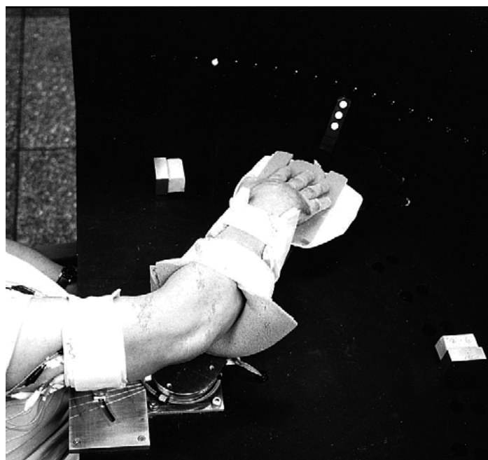
Fig. 2.5. Robotic Assistance of Upper Limb Exercise. The image depicts the orthoses, the contact points with the arm and the target towards which the lever should be aimed during extension and flexion of the elbow (Cozens, 1999).
