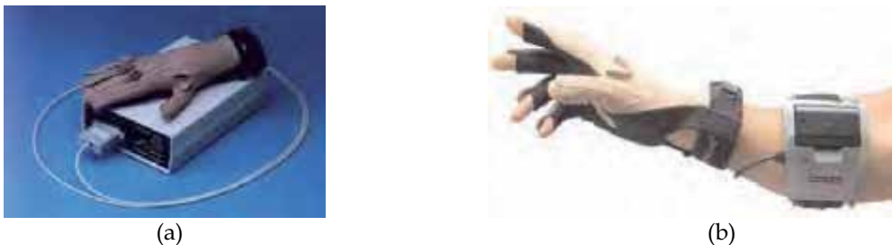
Fig. 3.3. The Cyberglove sensing Glove (a) Desktop version (b) Bluetooth wireless version. Picture Immersion Corporation.
