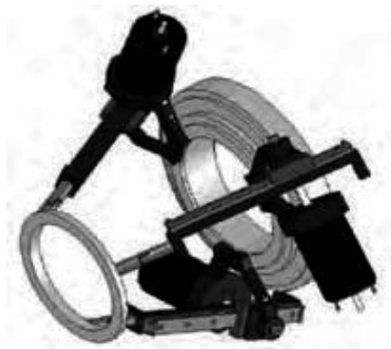
Fig 4. Wrist component of the MAHI arm exoskeleton employing electrical motors with a cable drive.
