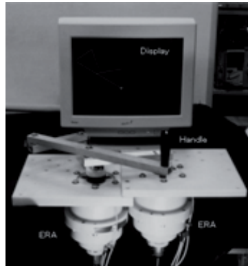
Fig. 4. Rehabilitation system “NIHO-1”.
