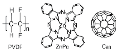
Fig. 11. Chemical structures of PVDF and ZnPc:C 60 donor-acceptor systems.
