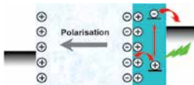
Fig. 10. A schematic display of an anode/ blocking layer /active layer/ cathode photosensor.
