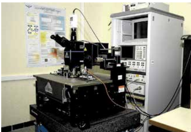
Fig. 19. RF probe station connected with a vector network analyzer
