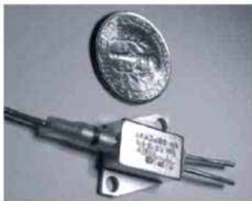
Fig. 18. The fiber-coupled output module from a single emitter.
