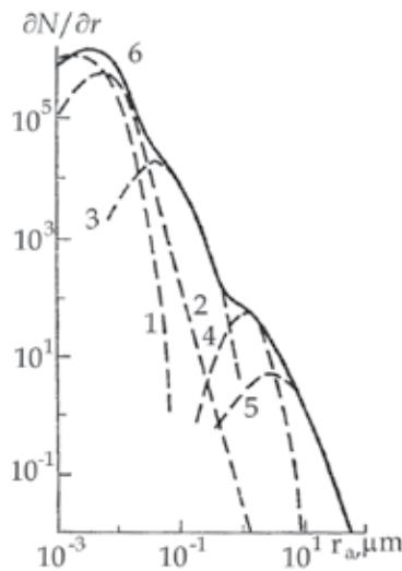
Fig. 22. An example of construction of model of microstructural characteristics (a curve 6) sooty ashes in the form of superposition of definitely weighed fashions curves 1, 2, 3, 4, 5.
