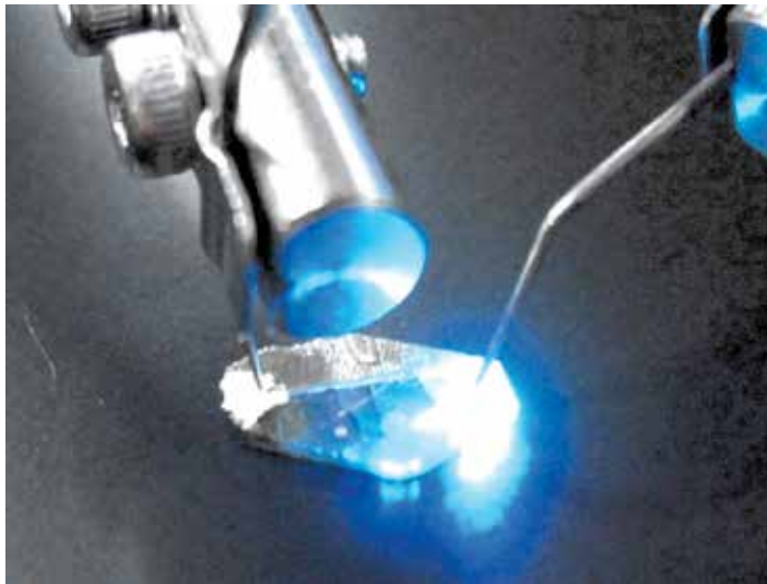
Fig. 8. Photograph of LEDs on a GaN wafer produced by the ammonothermal method.
