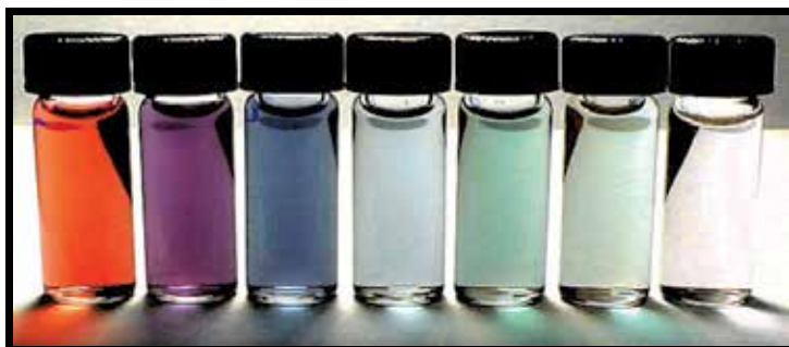
Fig. 24. The effect of size quantization: light emission from gold colloids with varying size of nanoparticles, smallest particles emit violet and the largest emit red color.
