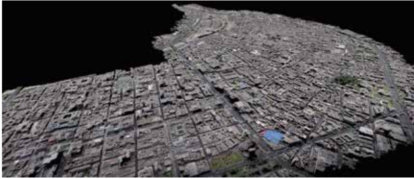
Figure 11. 3D point cloud produced with the drone to show building heights in BA. Source: ReMap Lima.
