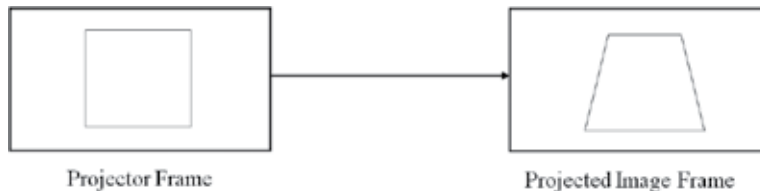
Figure 6. Projected image is distorted when projected onto an oblique surface.
