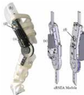
Figure 7. Proposed exoskeleton for knee assistance. (a) Rotary SEA module, (b) a thigh brace, (c) a calf brace, (d) a motor driver, (e) a DC motor, and (f) a controller (Kong et al., 2010).
