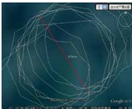
Figure 12. The minimum turning circle (radius 1.375 m).
