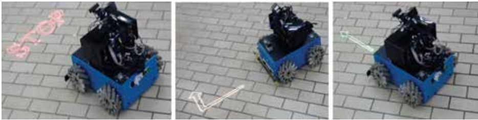
Figure 11. Laser notification to all interactants and LCD menus.
