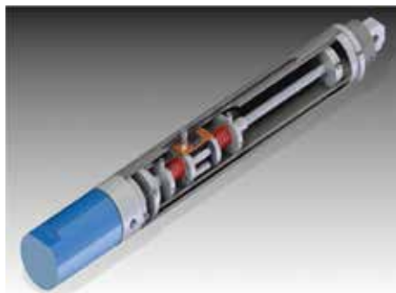
Figure 12. Actuator final design with internal components.
