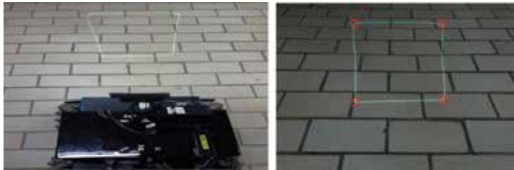
Figure 8. Projection of calibration target and corner extraction.
