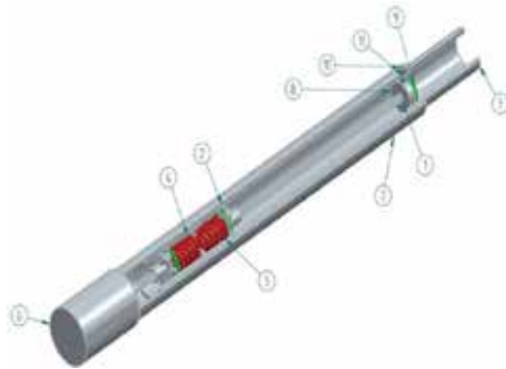
Figure 10. First prototype showing internal actuator components: ball screw (1); ball nuts (2); movable arm (3); springs (4, 5); motor & gearbox (6); base tube (7); bearing screw (8); O-ring (9); Allen screws (10); guide ring (11).
