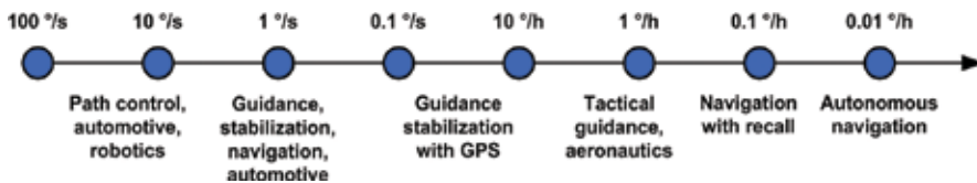
Figure 1. Bias instability of gyroscopes related to specified applications [16].
