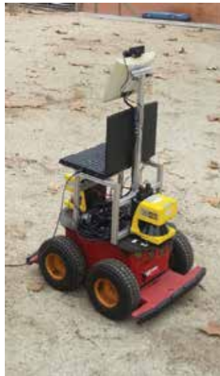
Figure 6. The robotic platform (based on the Pioneer 3 AT) used to capture the data sequences to test the described approach.
