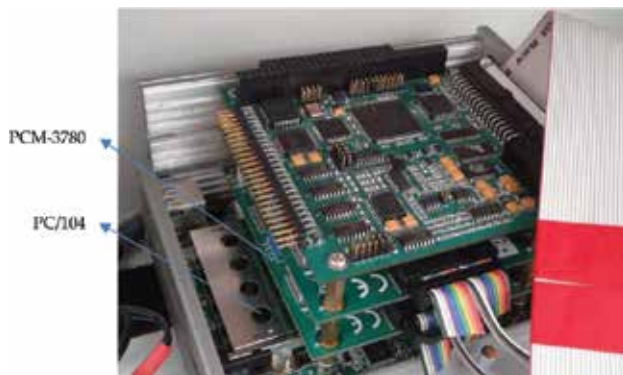
Figure 2. On-board control computer sub-system.
