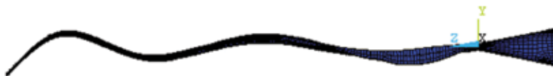
Figure 8. Bending mode following torsion mode of the 660 (kW) composite wind turbine blade.
