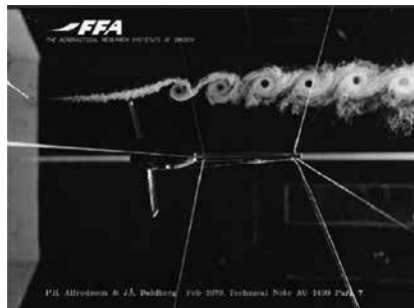
Figure 11. Visualisation of the tip vortices for the experiment done under non-yawed conditions by [42].
