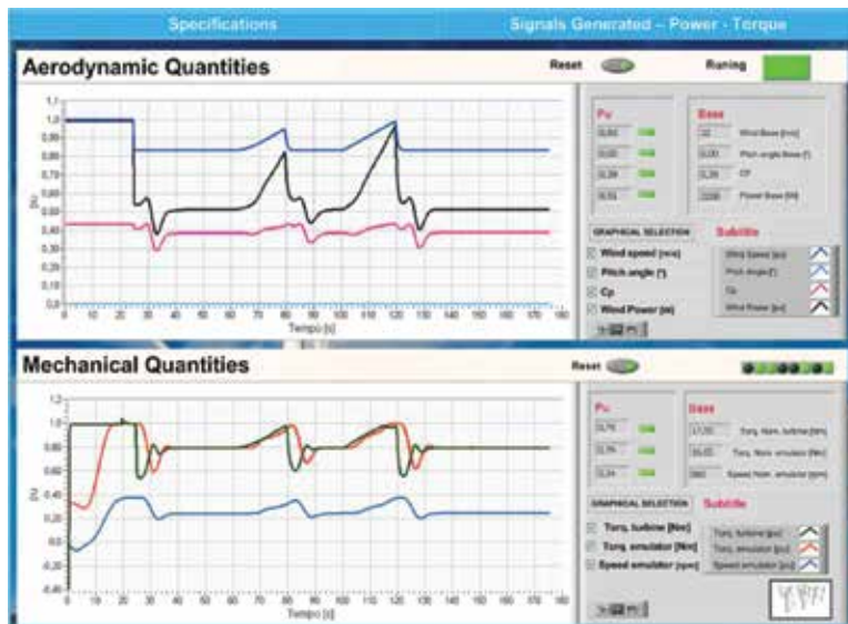
Figure 14. System emulator for the scenario with wind speed ramps.
