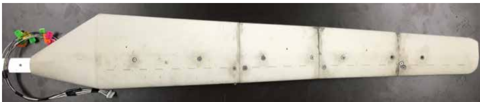
Figure 11. S809 wind turbine blade prototype with synthetic jet actuators.
