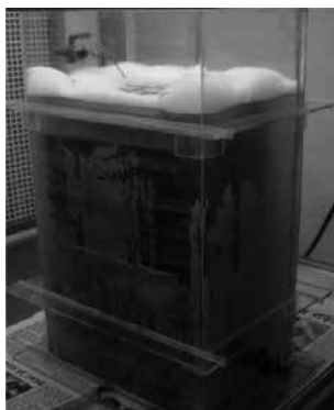
Figure 1. Picture of the biofilm-based packed bed bioreactor developed using the aerobic consortium BN7.
