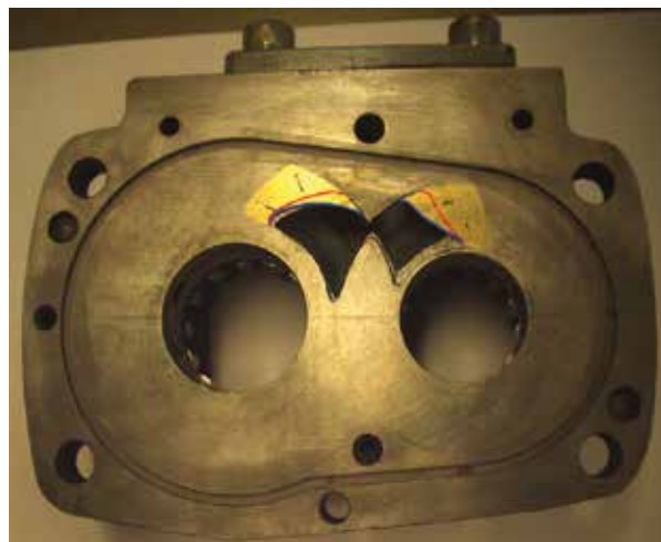
Figure 17. Modified shape of the discharge port.
