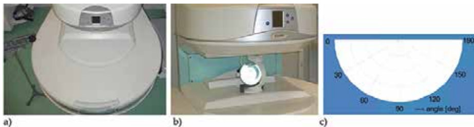
Figure 10. Arrangement photograph of the SPL distribution measurement in the MRI Opera neighbourhood with the sound level meter at the position of 30^\circ in the 45 cm distance from the middle point of the scanner (a), detailed photograph of the MRI scanning area with a testing water phantom inserted in the RF coil (b) and a principal angle diagram of the MRI scanning area (c).
