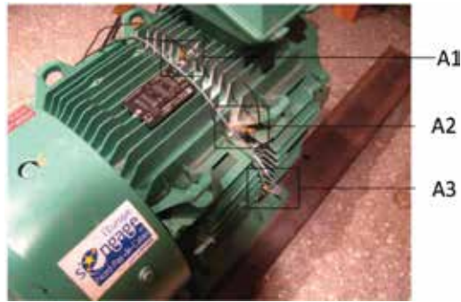
Figure 20. Positions of the accelerometers on M1.
