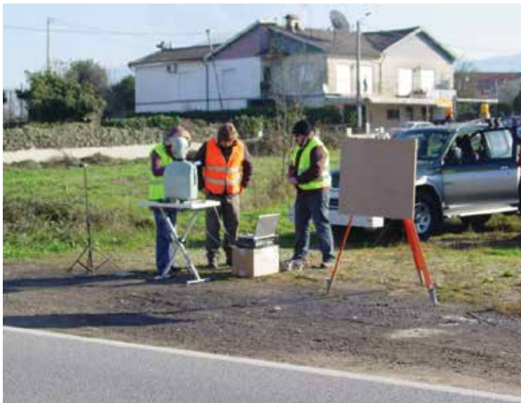
Figure 4. Measuring systems for SPB tests: microphone and HATS.
