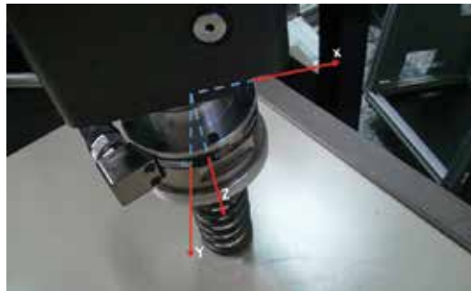
Figure 4. Robot's end-effector reference system equipped with the ATI force sensor and an elastic interface.
