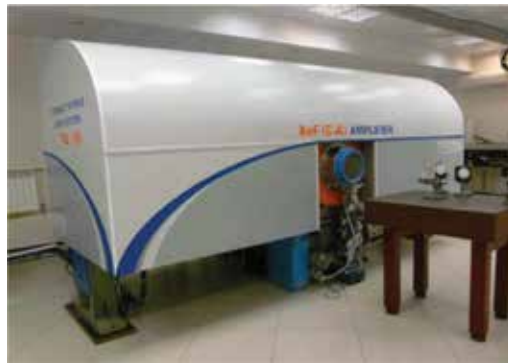
Figure 8. General view of the XeF(C-A) amplifier.
