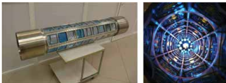
Figure 9. (a) Laser cell of the XeF(C-A) amplifier. (b) Inside view of the laser cell with the mirror unit.
