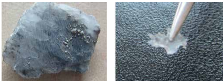
Figure 9. Thin film of hydroxyapatite on the salt after heated/thin and flexible film of HA.
