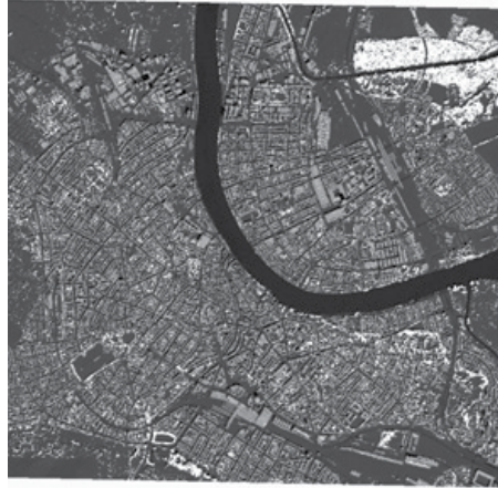
Figure 10. DART reflectance image for an NIR band (864.6 nm), over the city of Basel, corresponding to a Landsat-8 image, with erroneous (but realistic) optical properties used as input.
