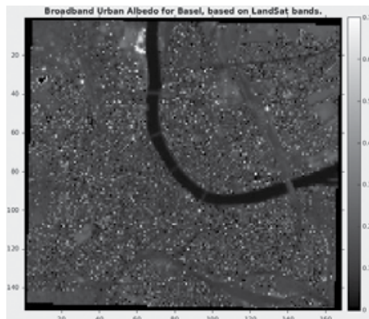
Figure 11. Urban surface albedo image computed using the direct calibration method for the city of Basel, with a Landsat-8 multispectral image.
