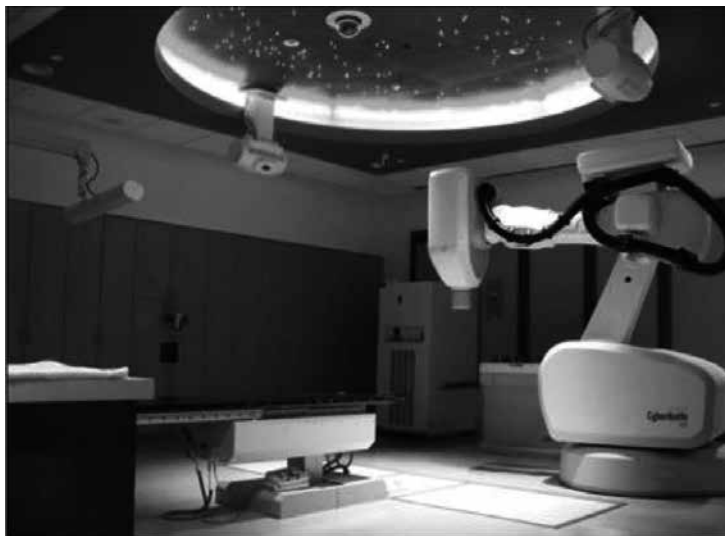
Figure 6. The Cyberknife VSI system installed in a clinical setting. Note the two X-ray tubes mounted on the ceiling and the X-ray detectors that are placed beneath the floor of the treatment vault for stereotactic imaging and on-line tracking.
