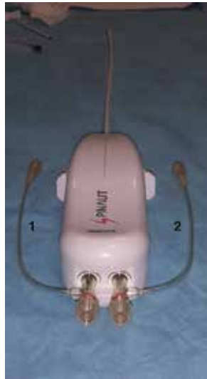
Figure 13. Fiberoptic camera advances from the left input (1), laser probe advances from the right input (2).
