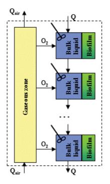
Figure 6. Structure of trickling biofilter [7].
