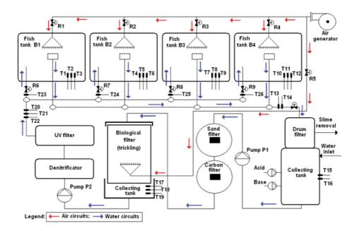
Figure 3. Experimental plant of the recirculating aquaculture system [4].
