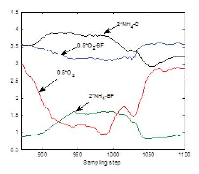
Figure 15. Evolutions of ammonia concentrations at biofilter input and output,  $NH_4$ -C and  $NH_4$ -BF (mg/L) (black and green, respectively) and of oxygen concentrations at biofilter input and output,  $O_2$  and  $O_2$ -BF (mg/L) (red and blue, respectively).
