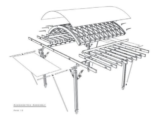
Figure 6. Assembly of the modular unit.
