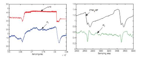
**Figure 17.** (a) Evolution of the level in the tank located after mechanical filter, L (cm), and of total inflow of the aquaculture tanks (filtered),  $IF_i$  (m<sup>3</sup>/h); (b) evolution of recirculating flow,  $IF_i$  (m<sup>3</sup>/h) affected by two consecutive washes of filters, together with the corresponding variation of ammonia concentration in biofilter NH<sub>4</sub>-BF (mg/L).
