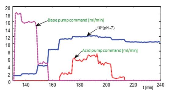
Figure 16. The response of pH control system.
