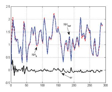
**Figure 11.** Validation of the identified model using adaptive filters (model output—blue line, output of the emulated process—red line and identification error—black line).
