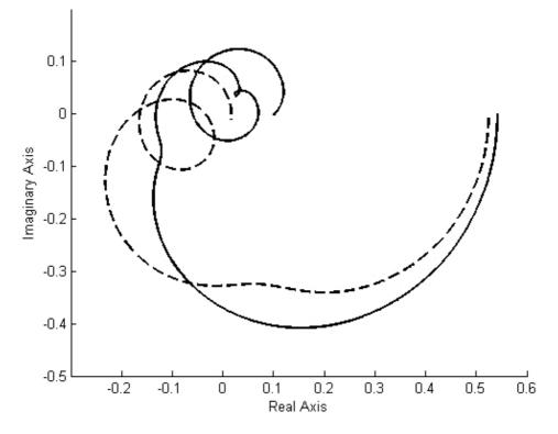
**Figure 13.** Nyquist frequency characteristic of the channel  $NH_{4,in}(t) \rightarrow NH_{4,out}(t)$  (regime high flow—solid line and regime low flow—dashed line).
