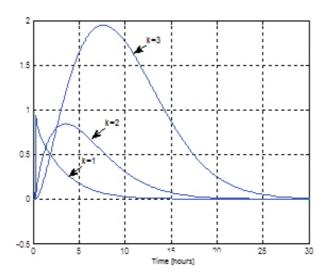
Figure 8. Pulse response of the elements k from the biofilter structure (the case of non-linear model).
