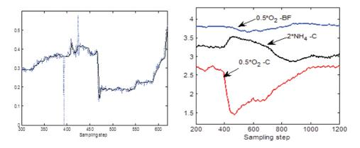
**Figure 14.** (a) Sample of ammonia concentration at the biological filter output,  $NH_4$ -BF (mg/L): unfiltered (dot) and filtered signal (solid); (b) evolution of ammonia concentration at the biofilter input,  $NH_4$ -C (mg/L) (red) and of oxygen concentrations at the biofilter input and output, respectively,  $O_2$  and  $O_2$ -BF (mg/L) (red and blue, respectively).
