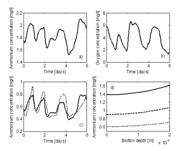
**Figure 10.** Simulation results of the identified model of trickling biofilter: (a) ammonia concentration in the influent; (b) dissolved oxygen concentration in the influent; (c) ammonia concentration in the effluent (experimental data—dashed line, evolution of the identified model—solid line); and (d) ammonia concentration along the biofilm thickness (Zone 1—solid line, Zone 3—dotted line and Zone 5—dashed line) [10].
