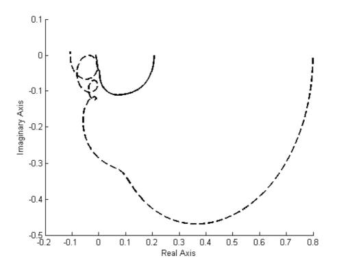
**Figure 12.** Nyquist frequency characteristic of the channel  $Q_{in}(t) \rightarrow NH_{4,out}(t)$  (regime high flow—solid line and regime low flow—dashed line).
