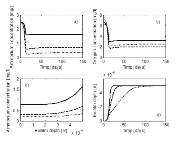
**Figure 9.** Simulation of the analytical model of trickling biofilter (Zone 1 – solid line, Zone 3 – dotted line and Zone 5 – dashed line): (a) ammonia concentration in liquid volume; (b) dissolved oxygen concentration in liquid volume; (c) profile of ammonia concentration along the biofilm thickness; and (d) evolution of the biofilm thickness in trickling biofilter [10].
