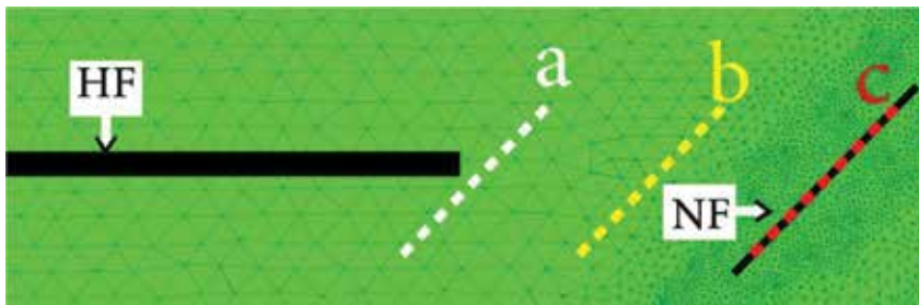
Figure 5. Areas of study for debonding investigation when natural fracture with a 45° angle relative to the hydraulic fracture spread.
