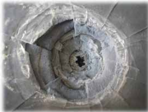
Figure 13. Crater originated in the double ceramic plate.
