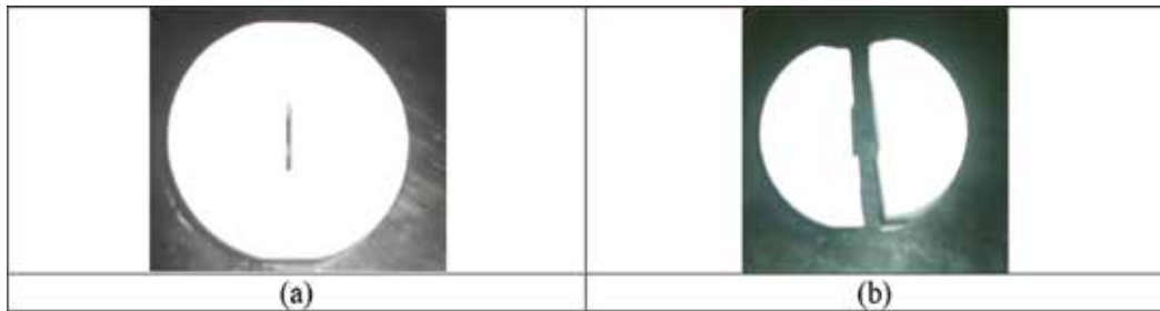
Figure 15. (a) CSTFBD before testing and (b) failure mode of CSTFBD specimens.
