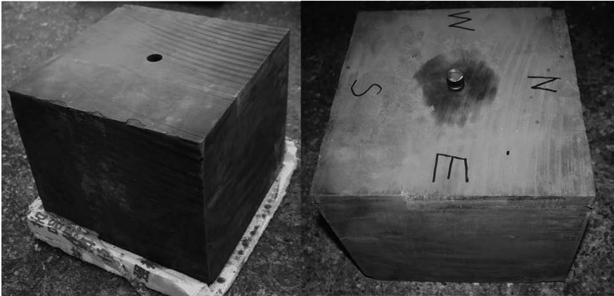
Figure 2. The shale specimen for hydraulic fracturing test.
