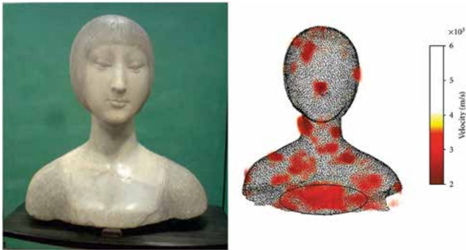
Figure 13. 3D ultrasonic travel time tomography on the Eleonora d'Aragona statue. Adapted from Cosentino et al. [4].
