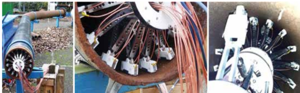
Figure 29. LRU collar for pipeline monitoring.
