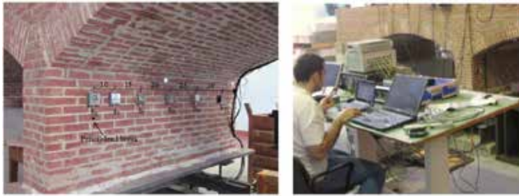
Figure 6. Wave velocity test: (left) the sketch of the pencil-lead break point and the sensor distribution and (right) scenario of the velocity test.
