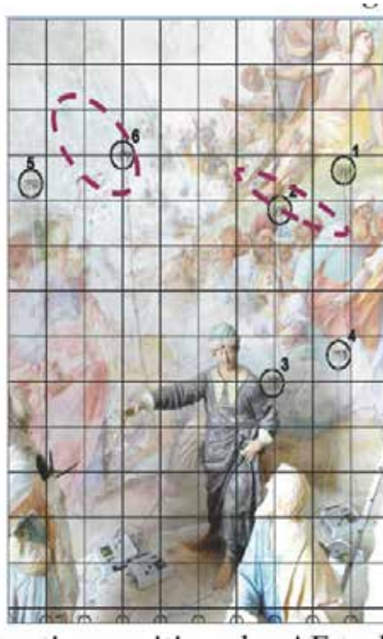
Figure 19. Monitored active positions by AE techniques are labeled by dashed lines.
