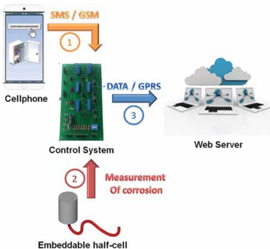
Figure 2. Design of the control system.
