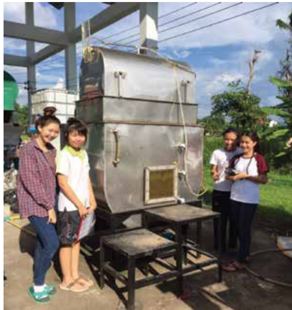
Figure 6. Wet fermentation (continuum type).
