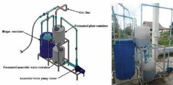
Figure 4. Dry fermentation anaerobic digestion process.
