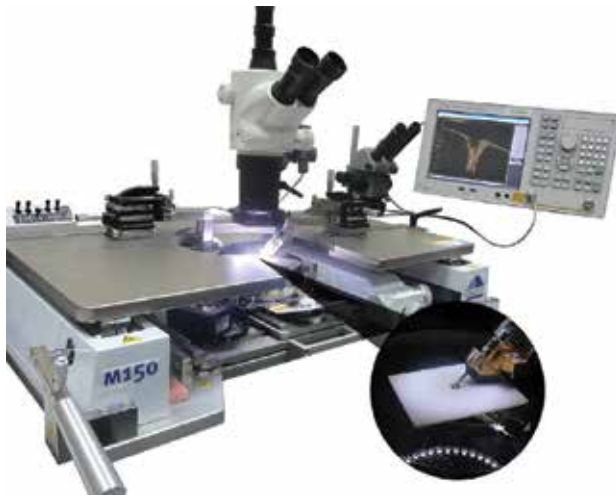
Figure 6. Experimental setup: E5071C network analyzer, M-150 probe station, and studied diamond-based PLS.
