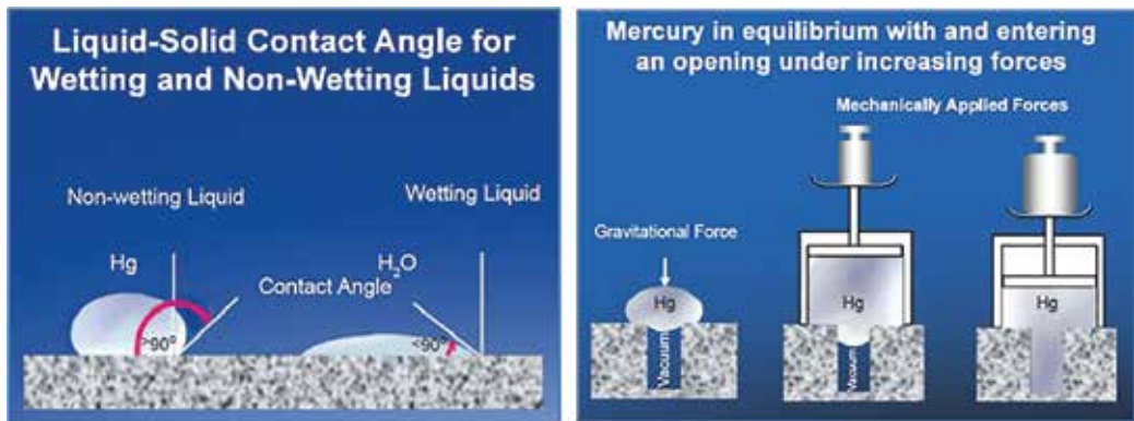
Figure 3. Left: different angles of contact for wetting and non-wetting liquids. Right: mercury (not-wetting liquid) does not penetrate pores by capillary, but it must be forced into them by the application of external pressure [9].
