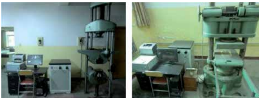
Figure 2. Wt60 t Universal Bending Test Machine and 200 t Compression Testing Machine.
