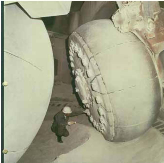
Figure 6. A view from the interior of a vertical roller mill.
