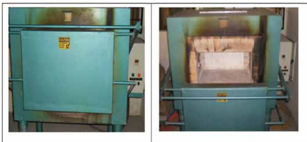
Figure 1. Automatic electric furnace used to heat concrete specimens.
