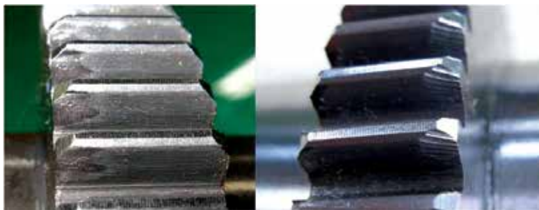
Fig. 8. Gear tooth weaned by misalignment
