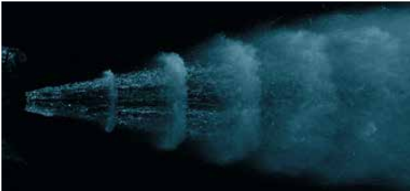
Fig. 12. The instantaneous structure of the fan pulsating water jet generated at 20 MPa (illumination by pulsed laser, camera Nikon D70s)
