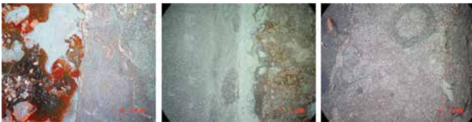
Figure 1. Macrographs of FSW (a), EBW (b), and GTA (c) welded AISI 4140 and AISI 304 subjected to molten salt environment at 600°C.
