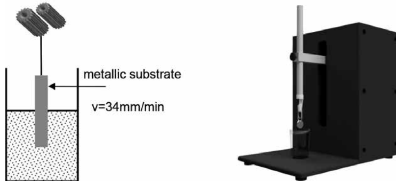
Figure 2. The scheme dip-coating process.
