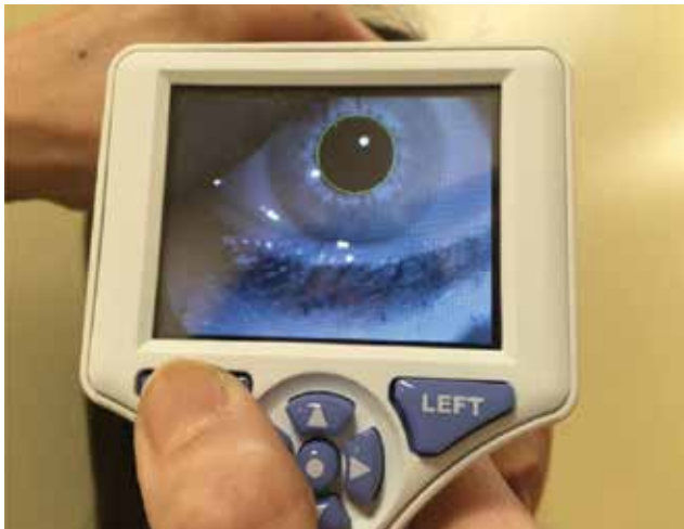
Figure 4. The NPi-200 Pupillometer (Neuroptics Inc, Irvine CA, USA, http://www.neuroptics.com ) uses quantitative infrared technology that objectively and accurately measures and trends the pupillary size and reactivity in critically ill patients. Eliminating inaccuracies caused by interpreter reliability. Measurement of NPi, (Neurologic pupillary index), maximal diameter at rest and maximal constriction as well as calculating % change and latency time between initiation of stimulation and onset of constriction. MCV, (maximum constriction velocities, mm/sec) is also calculated in each eye.
