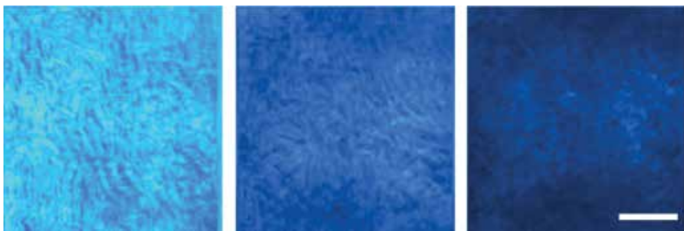
Figure 9. SHG images of a rabbit cornea at different depth locations (10, 100 and 100 \mu\text{m} ). The reduction in SHG signal is readily visible. This decrease in SHG effectiveness is mainly due to specimen-induced aberrations and scattering. Scale bar: 50 \mu\text{m} .
