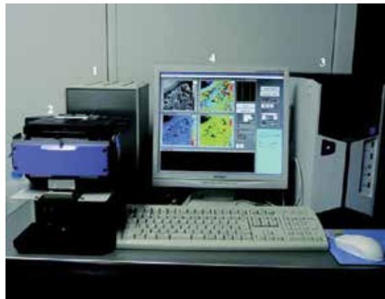
Figure 1. Appearance of scanning acoustic microscope systems. 1. Signal processor, 2. mechanical scanner with transducer, 3. system control PC, and 4. display.
