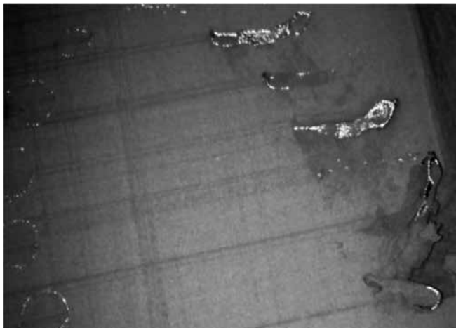
Figure 15. Selectively laser fusing the metal powder.
