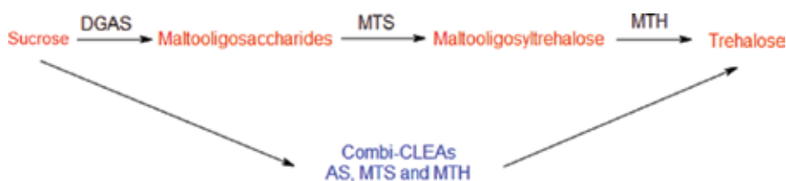
Figure 9. Biotransformation of sucrose to trehalose using combi-CLEAs in comparison to the use of individual enzymes for each reaction step.
