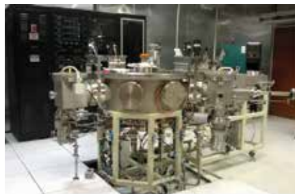
Figure 2. PECVD cluster tool from MVSystems, at the facilities of the Laboratory of Microelectronics of INAOE (project no. 152224 of the Secretary of Energy, SENER and the National Council of Science and Technology, CONACYT, Mexico).
