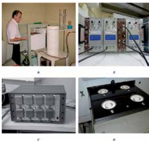
Figure 1. Equipment of a radioactivity laboratory: (A) \gamma -spectrometry; (B) \alpha -liquid scintillation (PERALS); (C) \alpha -Spectrometry (PIPS detectors); and (D) \beta -spectrometry (gas proportional counter), drawer with ^{90}\text{Y} oxalate sources.
