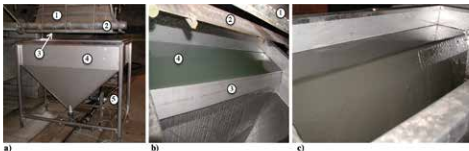
Figure 1. Irradiation dispositive used to irradiate sludge. (a) Overall view of the system, showing the accelerator scanner (1), the window blower (2), the electron beam shutter (3), the sludge delivery system (4), and the pipes delivering the sludge to the system (5). (b) Simulation of the process using tap water. (1) Lower portion of the accelerator scanner, (2) beam shutter, (3) weir, and (4) incoming water. The depth of the sludge layer at the top of the weir was about 0.3–0.4 cm. (c) sludge sample (adapted from [7]).
