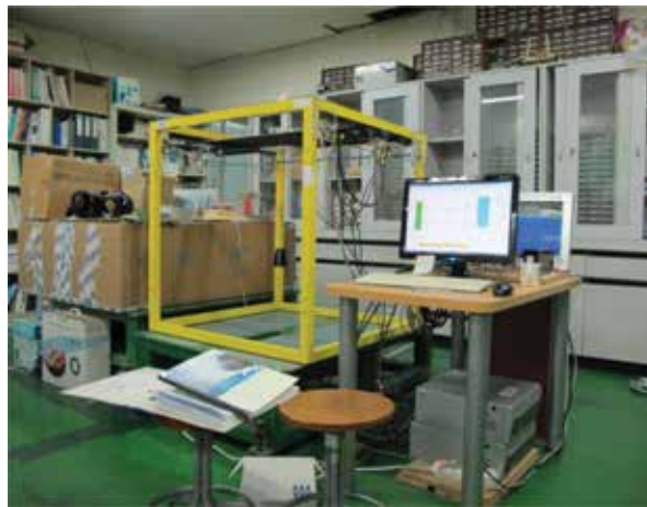
Figure 5. Overhead crane system used for the experiments.
