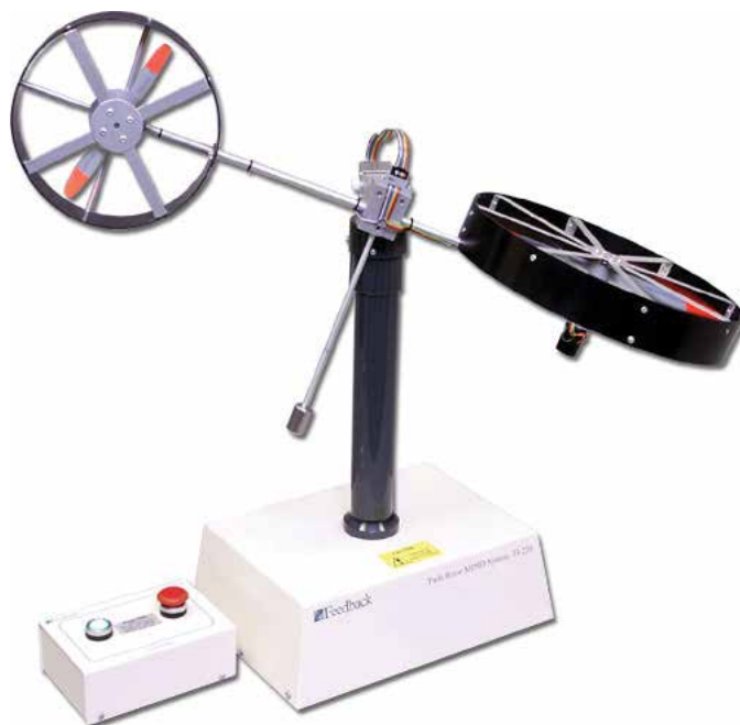
Figure 1. Twin rotor MIMO system.
