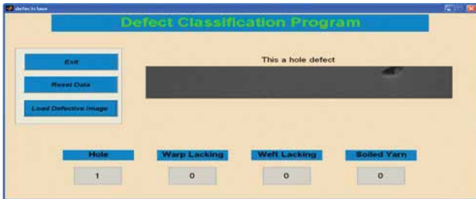
Figure 17. Classification of hole defect.
