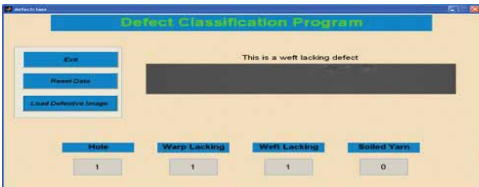
Figure 19. Classification of weft-lacking defect.
