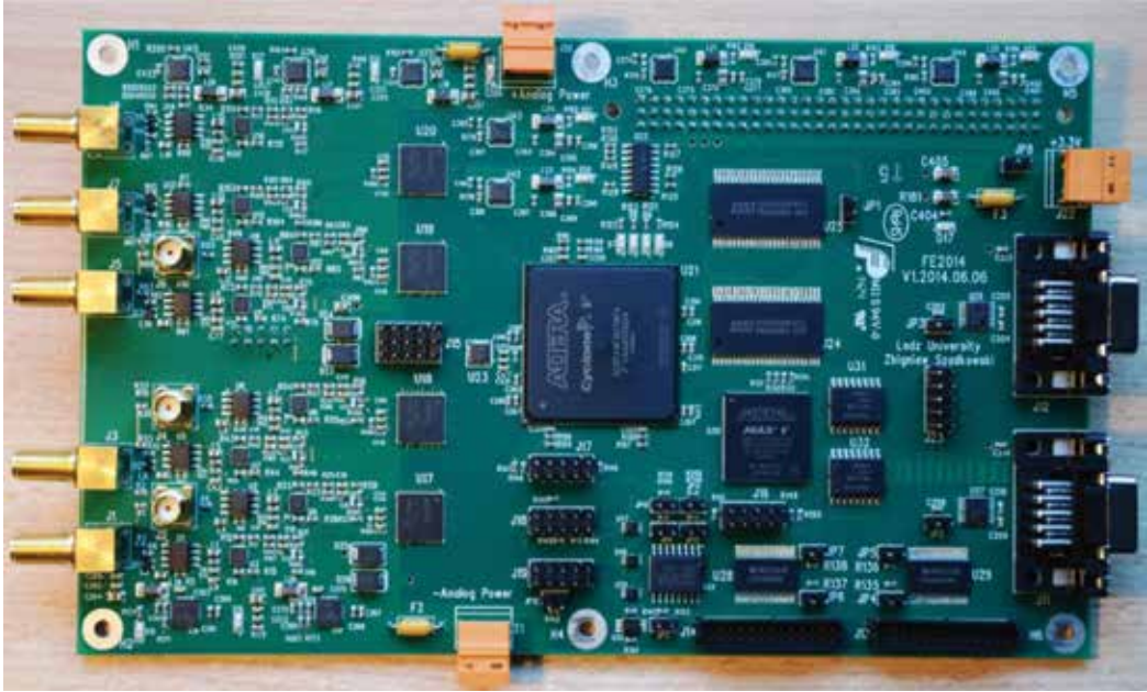
Figure 12. The front-end board with Cyclone V E FPGA used for high-resolution tests in the Pierre Auger Engineering Array.
