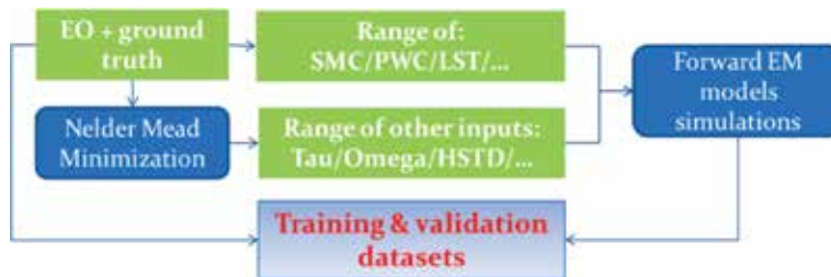
Figure 1. Strategy adopted for defining the training and validation datasets, starting from the experimental data and using the forward e.m. models (after [16]).
