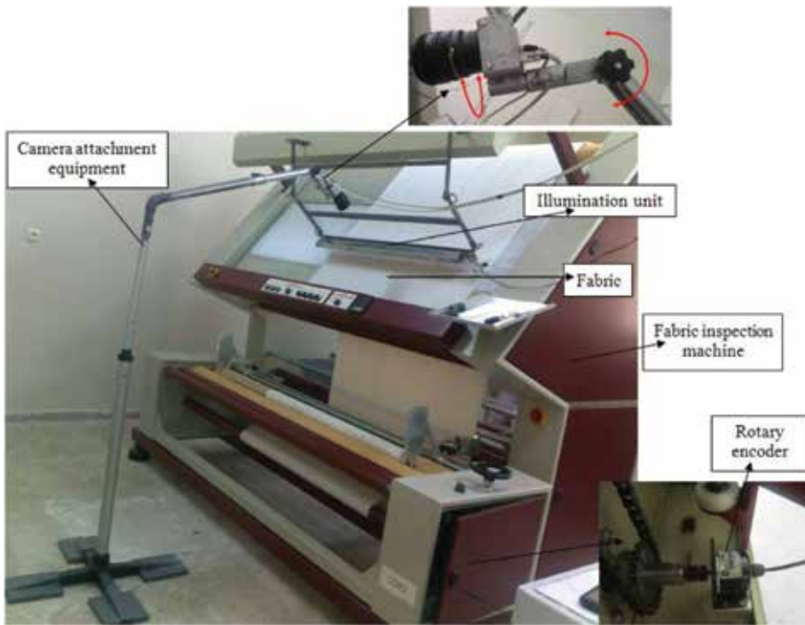
Figure 6. Machine vision system for fabric inspection.
