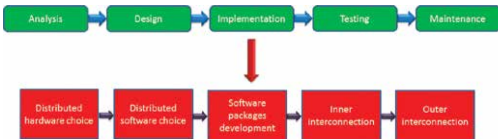
Figure 5. Waterfall model for software design and development tasks for middleware.
