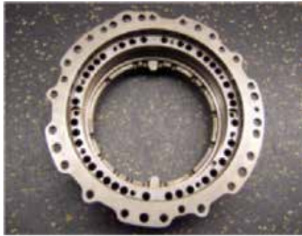
Figure 9. Laser repair technology of Titanium bearing housing [17].
