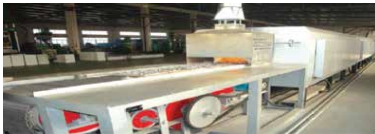
Figure 10. Mesh belt continuous resistance furnaces.
