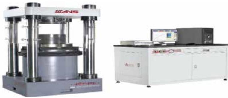
Figure 9. Isostatic compacting machine.
