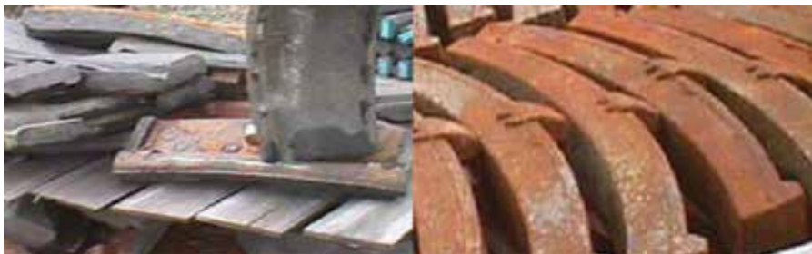
Figure 2. The cast brake shoes with wear indicators.
