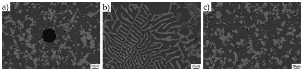
Figure 8. (a) Microstructure of metal matrix composite on the basis of EN HS 6-5-2/TetraC with large spherical pore, (b) and (c) structure of sintered at temperature 1300°C, (b) EN HS 6-5-2, (c) EN HS 6-5-2/TetraC.
