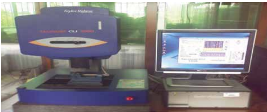
Figure 11. TALYSURF CLI 1000 equipment.
