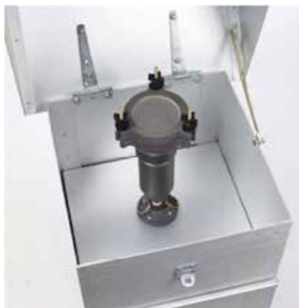
Fig. 2. Head of a PUF (polyurethane foam) sampler.
