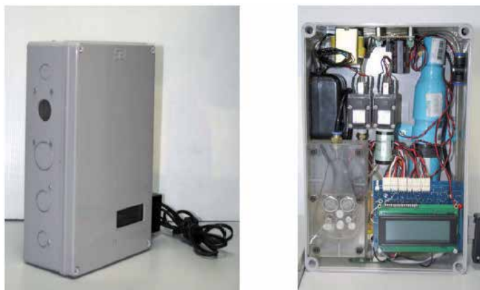
Fig. 18. Photographs of a wireless E-nose based on ZigBee wireless network (Pogfay et al., 2010).
