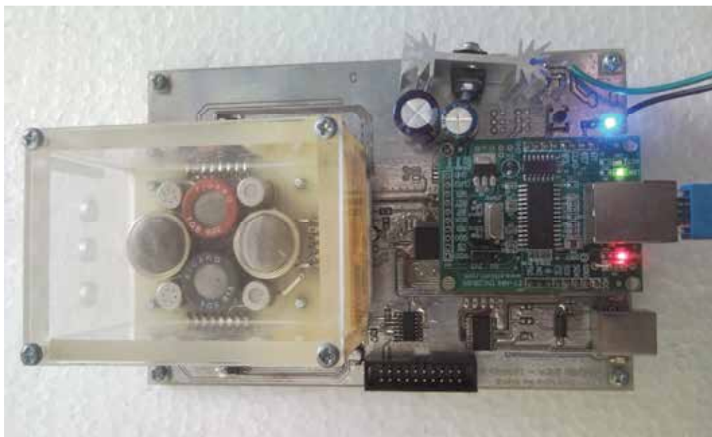
Fig. 17. Photograph of a networked E-nose (15 cm x 10 cm) developed by Center of Nanoscience and Nanotechnology, Faculty of Science, Mahidol University.
