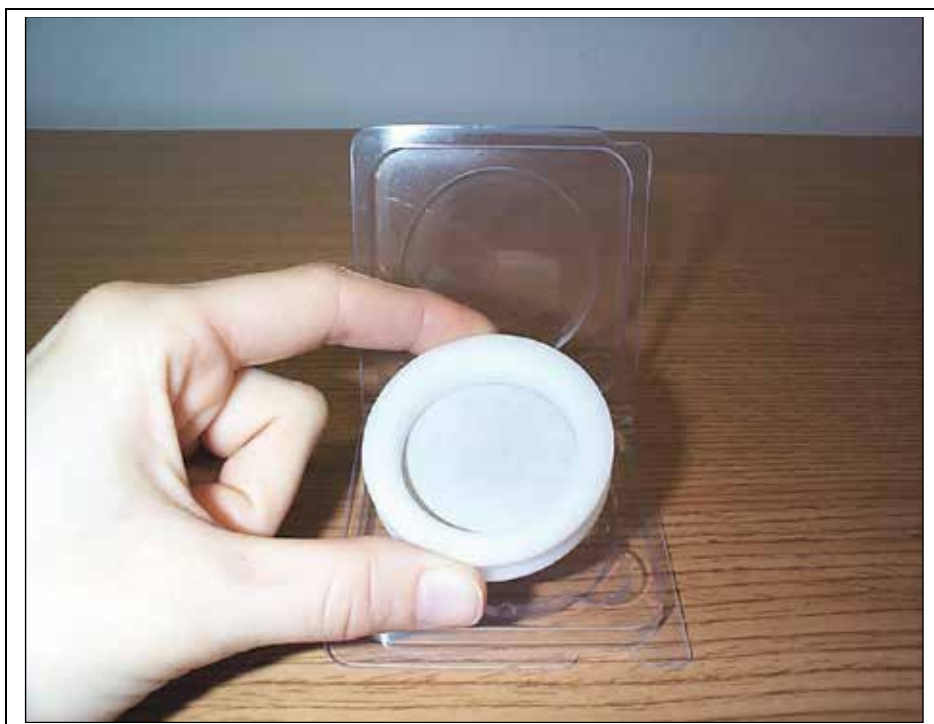
Fig. 2. Teflon Filter (47mm) Oil Coated in Sampling Cassette with Shipping Container (Ready for Field Use)
