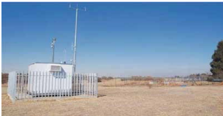
Fig. 6. Measuring station for taking particulate matter measurements Source: State of Air Report (2005)
