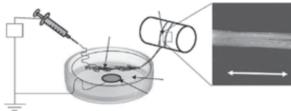
Figure 18. Schematic of the electrospinning setup used to obtain continuous self-assembled yarn structure [83].
