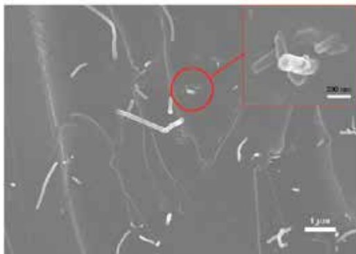
Figure 3. SEM rift image of the morphology of AG/MWCNTs UV-cured nanocomposite [6].
