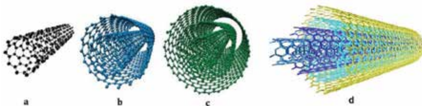
Figure 1. Schematic illustration of (a) SWCNT, (b) DWCNT, (c) TWCNT, and (d) multi-walled carbon nanotube (MCNT) [25].
