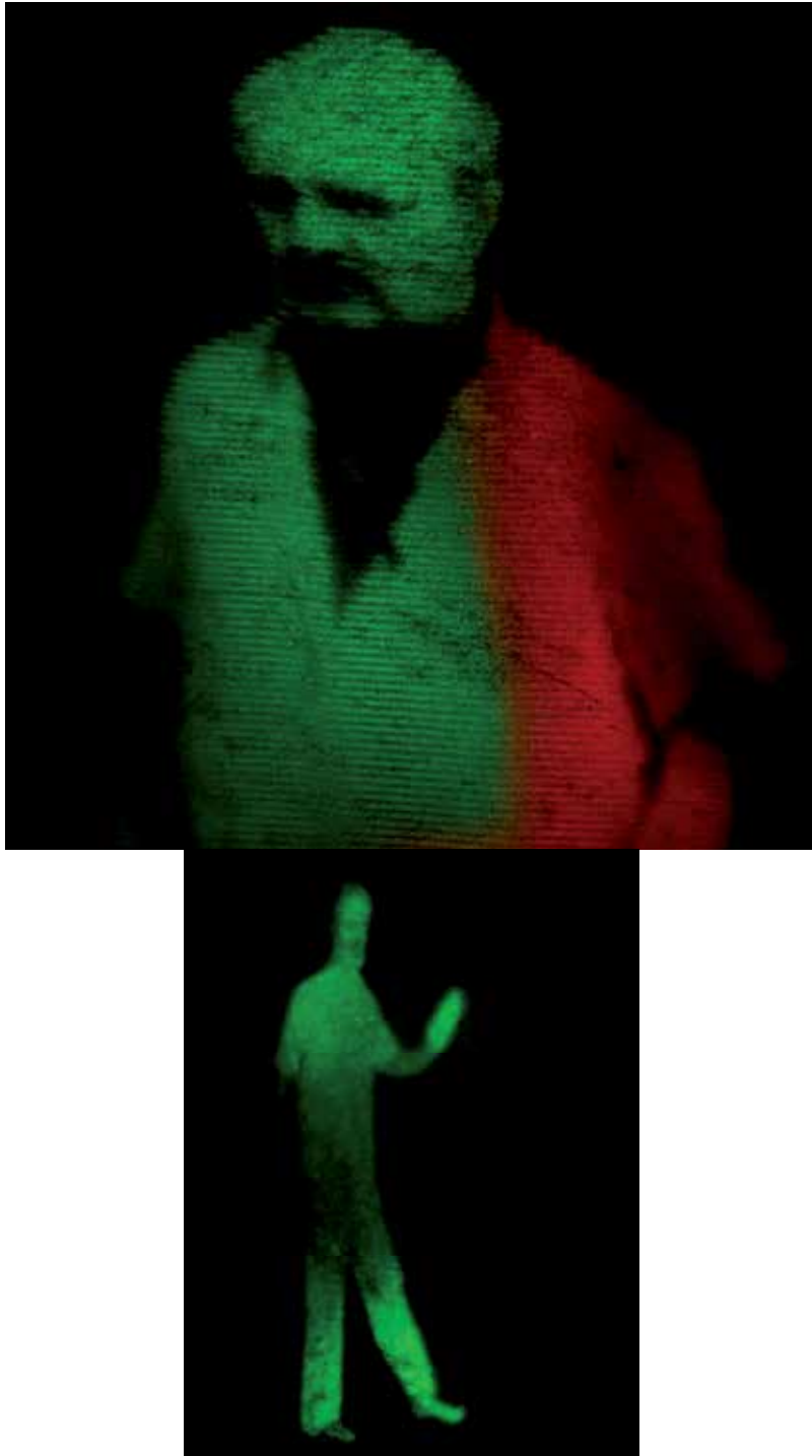
Fig. 8. Video scene appearing in an oblique plane in front of the screen. a) detail. b) complete image, 80 cm high, made of two hundred video lines.
