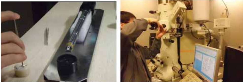
(d) The TEM grid is fixed on the specimen chamber.
