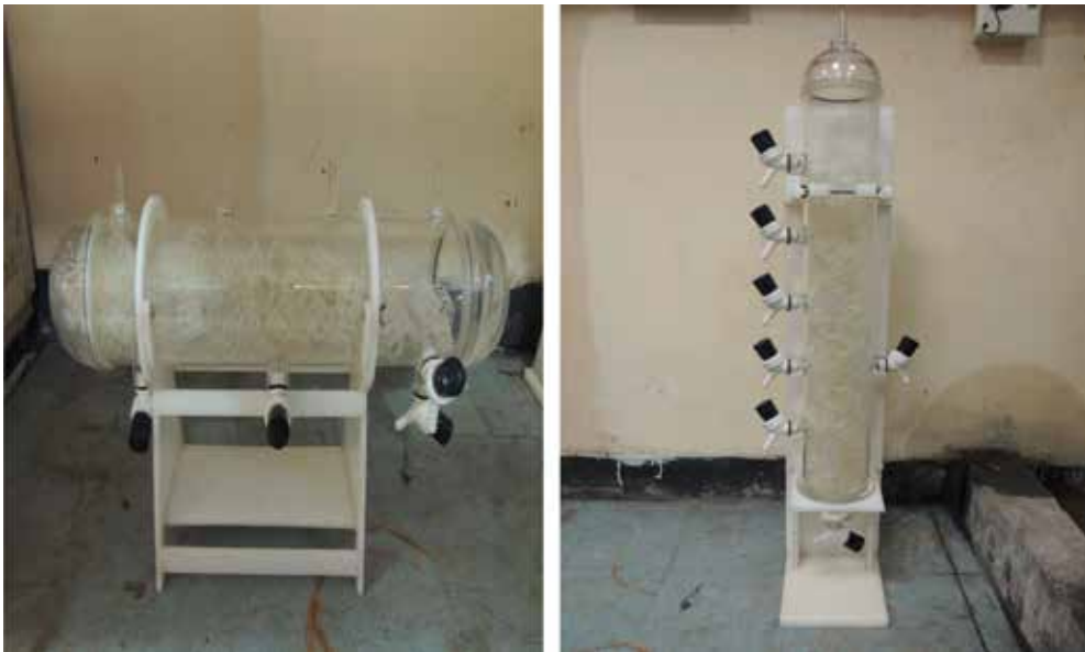
Figure 10. (a) Modified design of packed bed bioreactor. (b) Actual bioreactors constructed using plastic material.
