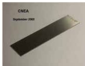
Figure 18. \gamma -U7Mo/Zry4 finished mini-plate of 100 x 25 x 1 mm 3 size. Meat and cladding thickness are 0.50 and 0.25 mm, respectively.
