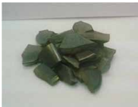
Figure 1. Eight millimeters thick uranium molybdenum lumps with residual stresses.
