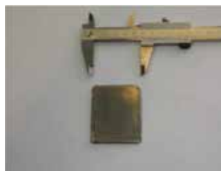
Figure 17. TIG welded sandwich of monolithic U7Mo meat and Zry-4 clad ready for hot co-lamination.
