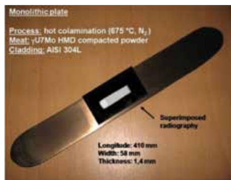
Figure 14. Monolythic UMo miniplate with stainless steel cladding.
