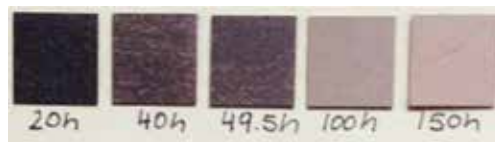
Figure 9. Expanded view of the 530°C gradual transition from black to grey oxide.
