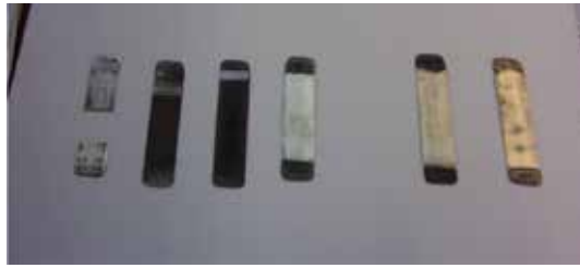
Figure 15. Monolithic \gamma -U7Mo/Zry-4 miniplates used along the different development stages. The three at the right extreme are in an intermediate step of surface oxide removal.
