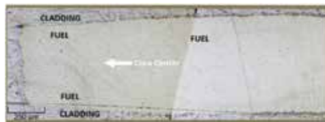
Figure 21. Metallographic cross-section of a hot zone in MZ50 miniplate.
