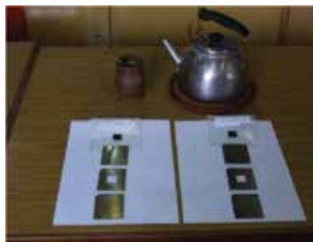
Figure 16. Finished frames, lids and coupons of MZ25 and MZ50 ready to be stacked and welded to conform the two sandwiches.
