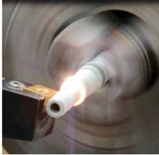
Figure 2. View of ceramics \text{Si}_3\text{N}_4 ( \text{Ø}14 \times 4.5 \times 104 \text{mm} ) heated by laser beam.
