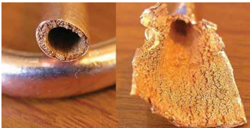
Figure 2. Metal sintered powder wick [15].
