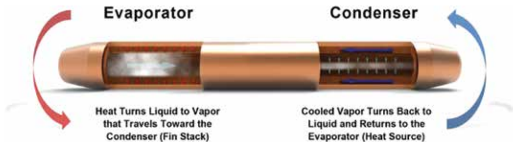
Figure 5. Cylindrical heat pipe [24].
