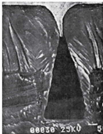
Figure 5. A vapor-deposited micro-grooved heat pipe [17].
