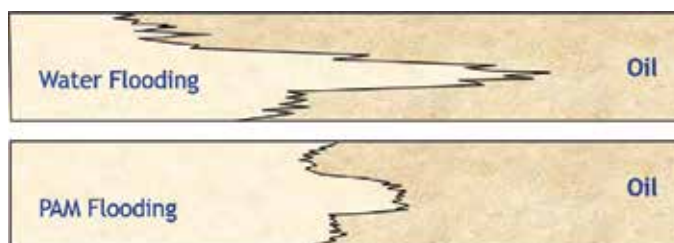
Figure 1. Water breakthrough can be delayed and sweep efficiency improved by increasing the viscosity of the injected fluid with polyacrylamide polymers (PAM) (modified with permission from Sorbie [11]).
