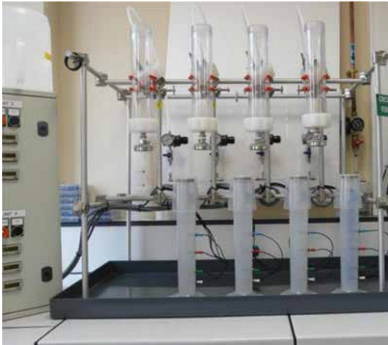
Figure 23. Typical set-up used to perform filter ratio tests with vessels (top) and graduated cylinders connected to a stopwatch (bottom) [25].
