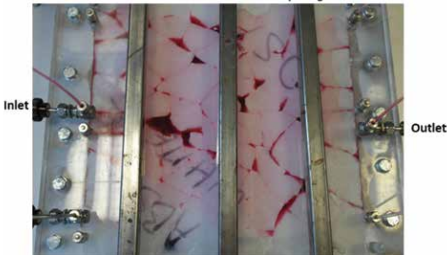
Figure 6. A square marble tile was fractured and reassembled within an aluminium frame sandwiched between two Plexiglas plates. The fracture network consisted mainly of narrow fractures with 12 large fractures. The vugular open fractures were larger bodies of open space varying between 0.4 and 2.2 cm aperture. These cavities were used to observe the advancing foam front during co-injection. In this figure, the marble tile model is filled with red-dyed brine to emphasize the fracture network.
