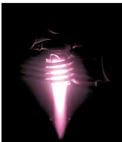
Fig. 1. Photograph of induction plasma generated by argon discharge
