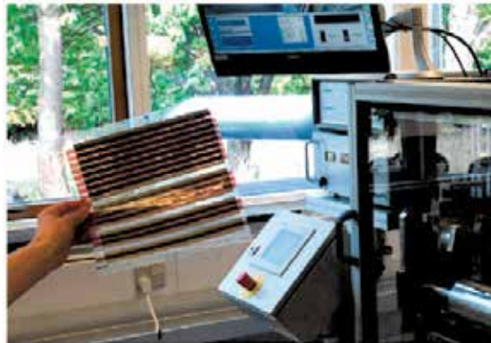
Fig. 12. Photograph of one of the final modules in front of the R2R coater. From Ref. (Krebs et al., 2009).
