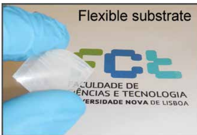
Figure 6. Photograph of \text{TiO}_2 nanostructured arrays on PEN substrates. All solvents produced similar samples, such as the one presented in this image.
