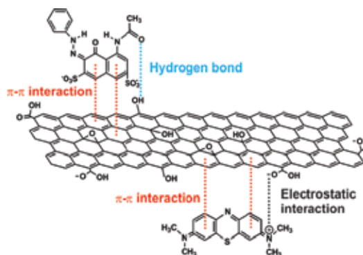
Figure 3. Scheme of interactions between RGO and AC1 dye molecules (up) and RGO and MB dye molecules (down). Adapted with permission from Kim et al. [27].
