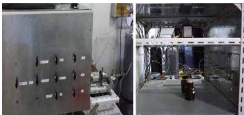
Figure 5. Images of the operating interface of reaction gas-dosing system for in situ DRIFTS test (©2014 Springer [18]).
