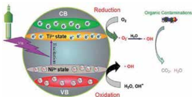
Figure 5. Schematic diagram of the photocatalytic process for Ni 2+ and Ti 3+ codoped TiO 2 under visible light irradiation [285].
