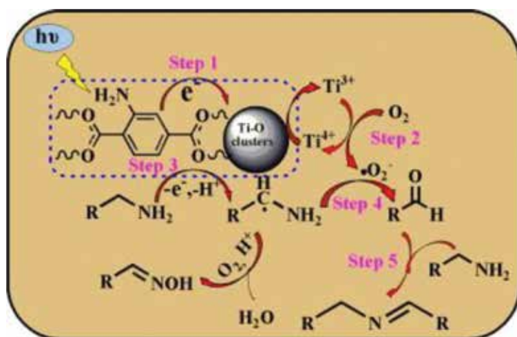
Figure 8. Suggested photocatalytic mechanism of the amines oxidation using NH_2 -MIL-125(Ti).
