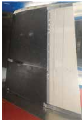
Figure 27. Complete CRIAQ wind tunnel test article including a morphing aileron [8].
