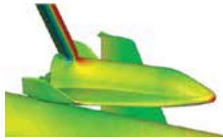
Figure 11. Sting effect on the old support. It is possible to see the red peak of pressure at the base of the sting; scale 1:180.
