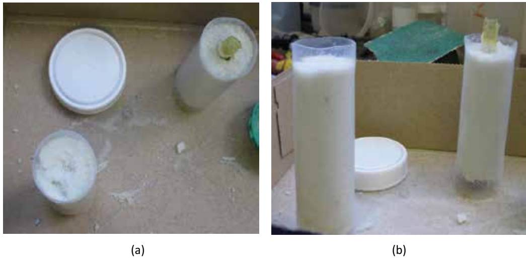
Figure 5. Preparation of synthetic rock samples (glass beads bonded with epoxy resins). (a) View 1 and (b) View 2.
