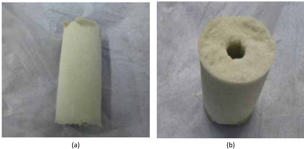
Figure 6. (a) A longitudinal view and (b) an oblique view of the synthetic rock (bonded glass beads).
