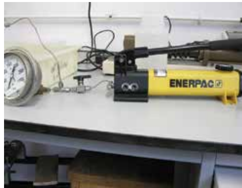
Figure 18. The manually operated hydraulic hand pump.
