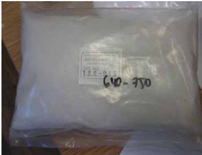
Figure 3. Graded glass beads a range of diameter between 640 and 750 \mu\text{m} .
