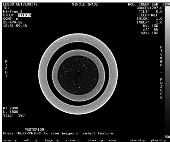
Figure 17. Scan image of the synthetic rock after collapse (high strength).
