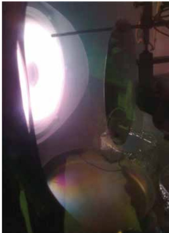
Figure 13. Typical RF sputtering process inside the vacuum chamber, under ultra-high vacuum conditions, to deposit platinum metal used for defining PRT and heater configurations.
