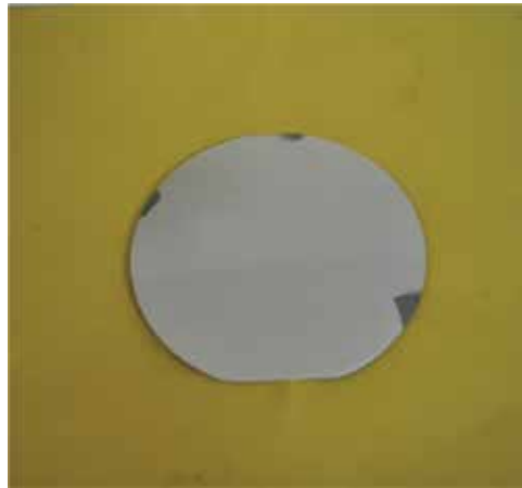
Figure 14. Photograph of platinum thin film deposited on oxidized three-inch-silicon wafer by RF sputtering technique.
