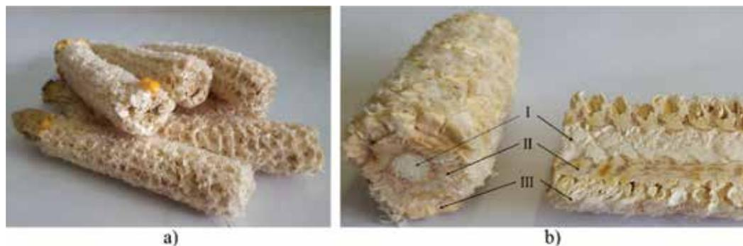
**Figure 2.** Corncob macrostructure: (a) general view and (b) longitudinal section [15].
