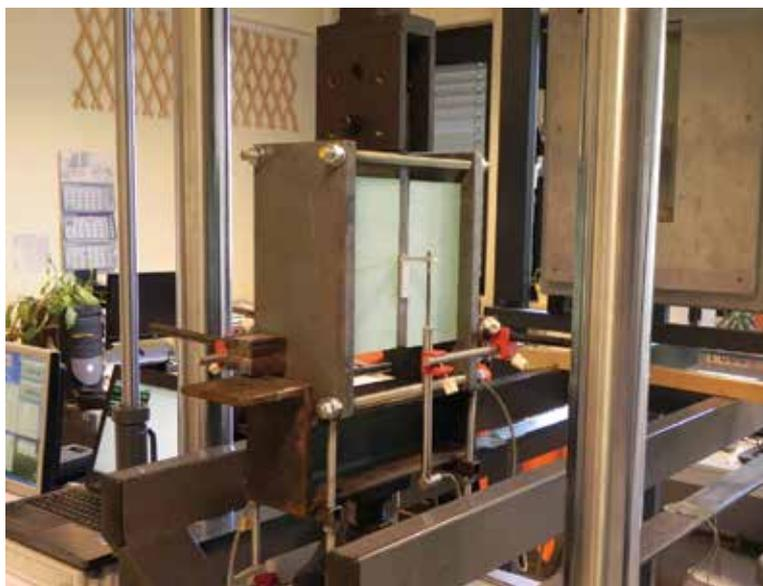
**Figure 5.** The XPS shear test setup.
