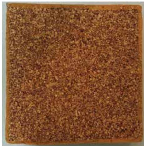
**Figure 11.** A sample of a 3-cm-thick corncob particleboard.
