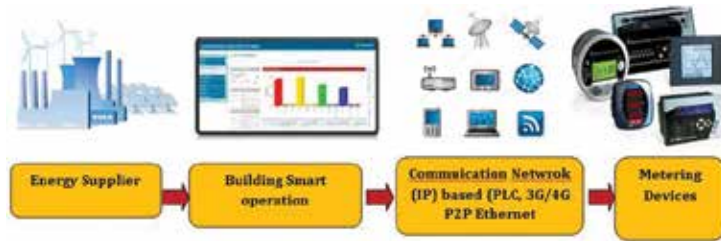
Figure 4. Flow chart for smart metering operations.
