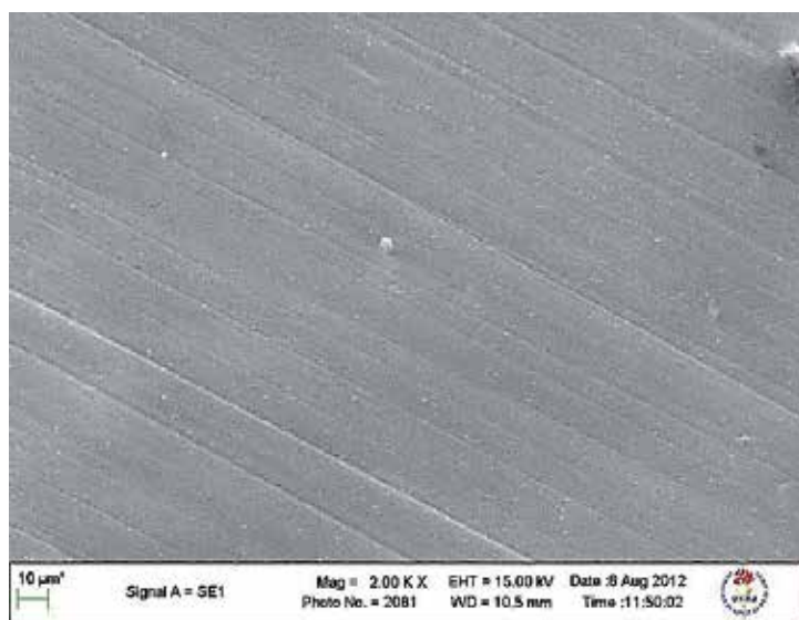
Figure 3. Surface morphology of Cu/ \gamma -Al 2 O 3 coatings produced at -1.20 V SSE from pyrophosphate bath previously stirred for 5 h at 800 rpm [61].
