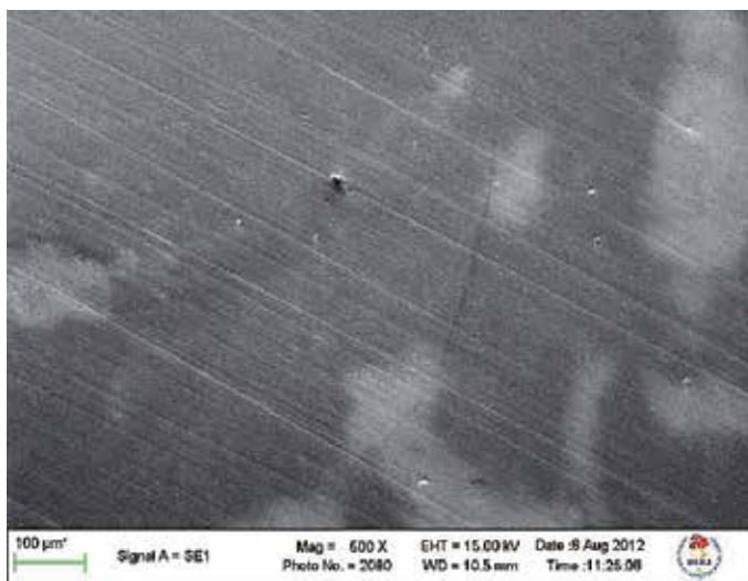
Figure 7. Surface morphology of Cu/ \gamma - \text{Al}_2\text{O}_3 coatings produced at -1.20 V_{\text{SSE}} from pyrophosphate bath previously stirred for 5 h at 800 rpm [61].
