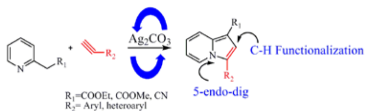
Figure 13. Silver-mediated oxidative C-H functionalization to synthesize indolizines [27]
